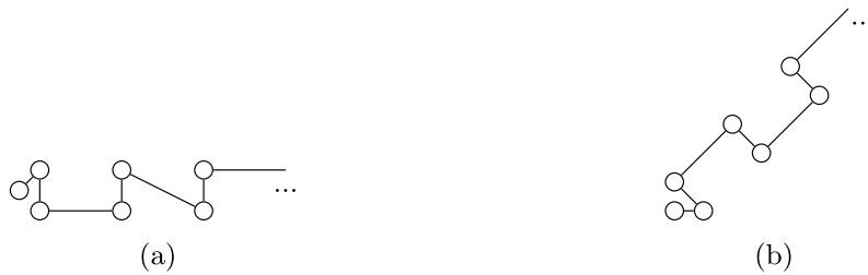
Fig. 11. Example of an undesired but optimal 1-path for a 2-chain before rotation (a). Papadimitrou's proposed optimal 1-path (in mode 2) after rotation (b).
